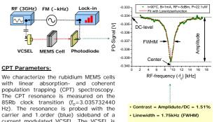
Hz). The resonance is probed with the carrier and 1.order (blue) sideband of a current modulated VCSEL. The VCSEL is • Center = 9.2 kHz (relative to f<sub>0</sub>) tuned to the D1-line (795nm)
